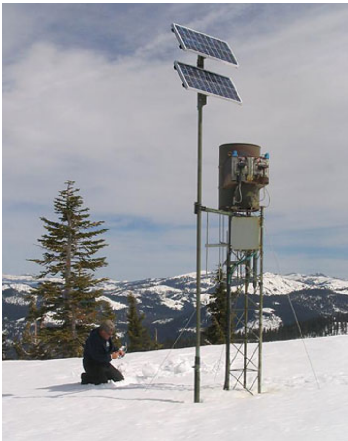
Cloud seeding generator in Nevada. Photo courtesy Desert Research Institute.
